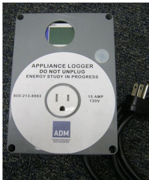
*Figure 3-2: ADM's Plug-In Appliance Logger*
