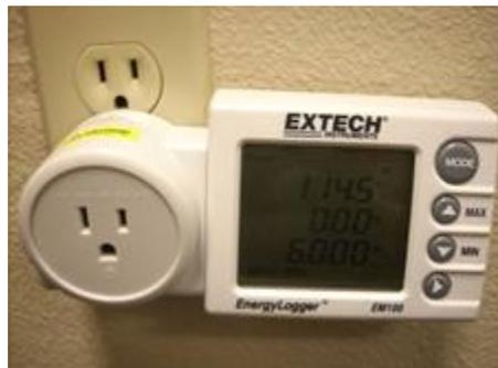
*Figure 6-1: Extech EM100 Plug-In Meter with Display*
