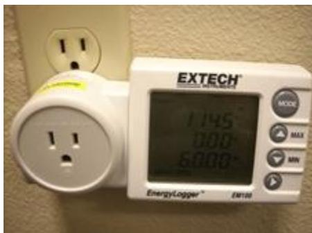
*Figure 3-3: Extech EM100 Plug-In Meter with Display*
