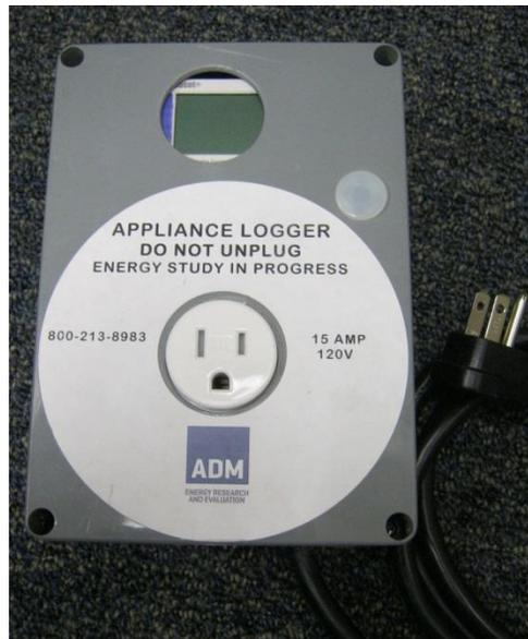
*Figure 6-2: ADM's Plug-In Appliance Logger*
