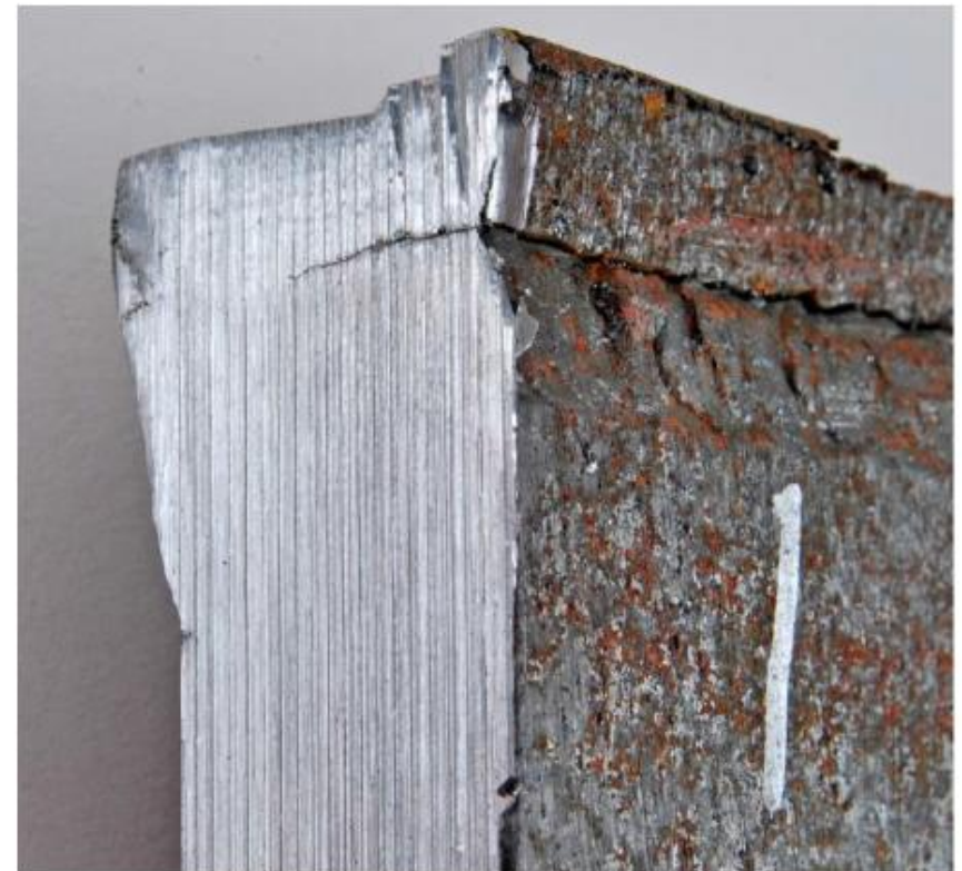
Figure 7 - Closeup of ID Initiated Crack
