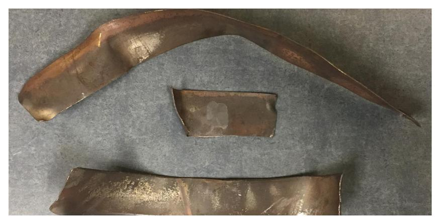
An employee found metal parts on the ground around Unit 1 stack while he was conducting his weekly rounds at facility. Unit 1 was taken out of service and a borescope inspection was conducted.
