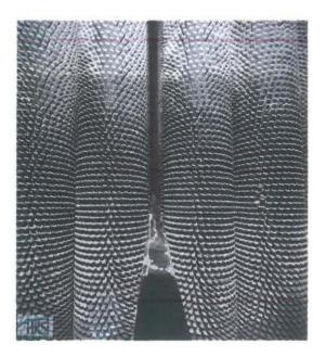
Figure 2.3 After Explosion Cleaning Front Row
