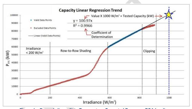
Figure 1 - Example linear fit to Temperature-Corrected Power vs. POA Irradiance
